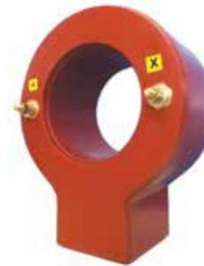
Damping reactors with cast-insulation are designed to limit commutation current of capacitor bank appearing at switching of capacitor bank (or some stages of capacitor bank) into electric network. Damping reactors are installed in a capacitor bank in series with power factor high-voltage capacitors.
